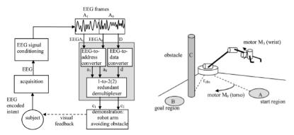
Controlling several robot motors using single EEG channel
